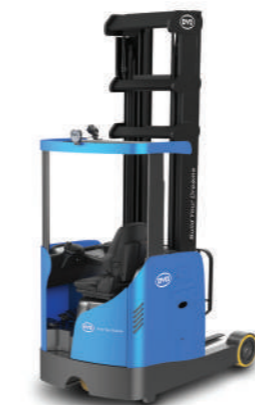
RTR16 Load capacity: 1.6 ton Service weight: 4,270 kg Voltage: 80 V Battery capacity: 270 Ah
