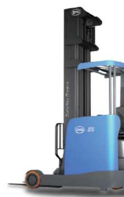
R20P Operation: Seat Load capacity: 2.0 ton Service weight: 4,550 kg Voltage: 80 V Battery capacity: 270 Ah
