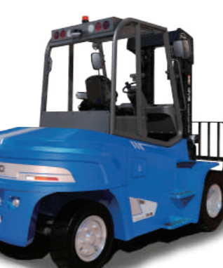
ECB60 Load capacity: 6.0 ton Service weight: 11,800 kg Voltage: 80 V Battery capacity: 1,080 Ah
