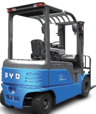
ECB30 Load capacity: 3.0 ton Service weight: 4,840 kg Voltage: 80 V Battery capacity: 270Ah/540Ah
