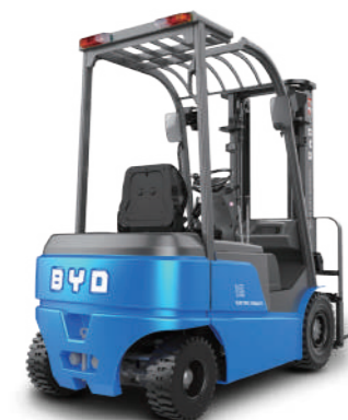
ECB16S Load capacity: 1.6 ton Service weight: 3,100 kg Voltage: 80 V Battery capacity: 270 Ah
