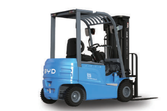
EL20-PRO Load capacity: 2.0 ton Service weight: 3,550 kg Voltage: 80 V Battery capacity: 210/270/420/540 Ah
