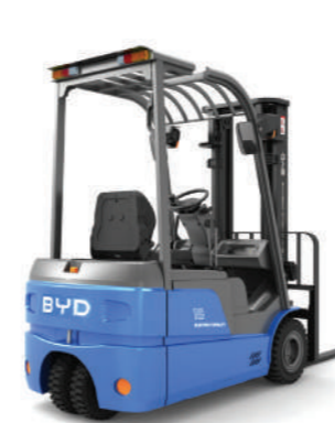
EL16-PRO (3 wheels) Load capacity: 1.6 ton Service weight: 3,100 kg Voltage: 80 V Battery capacity: 210/270 Ah
